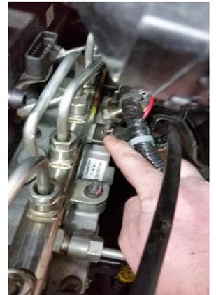
5. Remove bolt that holds dipstick tube in place.
