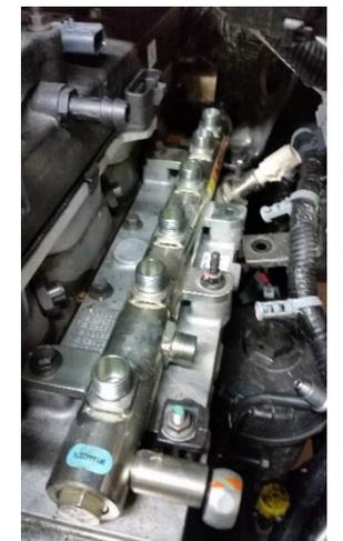
9. Unplug rail pressure sensor connector (located on the back of the rail near the firewall)
