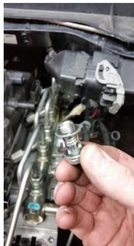
8. Remove all six injection lines starting with injection line #1
