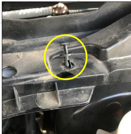
Figure 10: Remove plastic fastener
