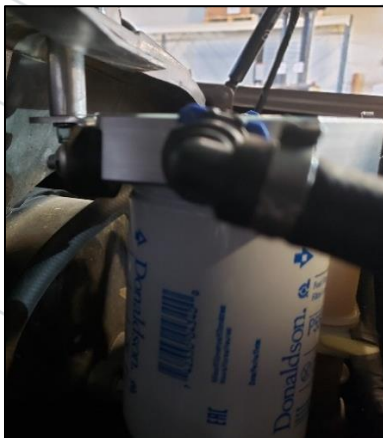
Figure 11: Spacer below cowl
