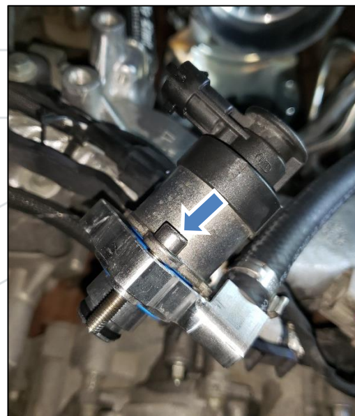
Figure 11: Subassemble Block, FCA, and front bolt
