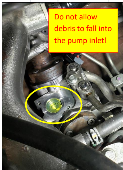
Figure 9: FCA Removed (no debris)
