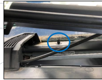
Figure 9: Clip under the cowl x2
