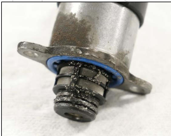
Figure 7: Failing CP4 FCA without Bypass Kit installed
