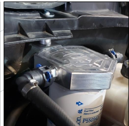
Figure 12: Filter Head Installed – 2017+
